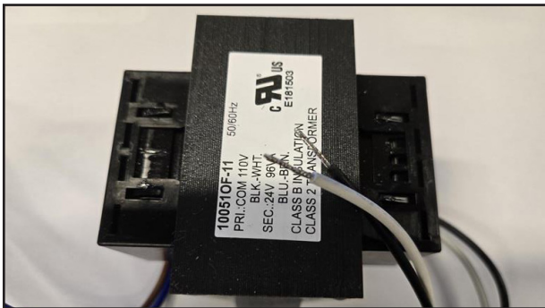
120 to 24VAC Transformer
