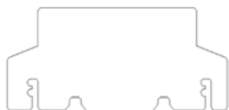
Restrictor plate for Set 1, Set 2 (Part # 761-060F)
