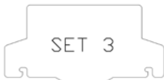
Restrictor plate for Set 3 (Part # 761-143F)
