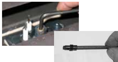
Diagram 2: Slide burner assembly to the right—then remove.
