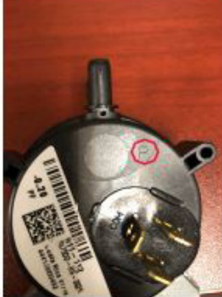
Pressure switch side "P"
