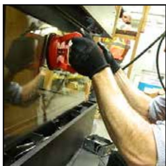
Handle glass with supplied vacuum clamps
