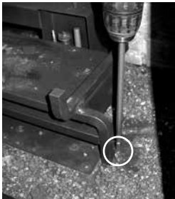
Diagram 1: Remove the left and right screws.
