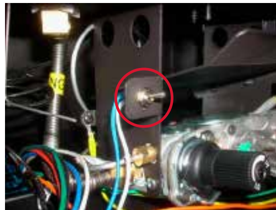
The Surefire switch is located above the valve. This can be accessed by removing the bottom louver/panel.
