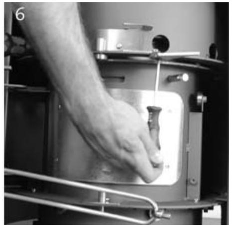
**Cleaning between the fixed part of the stove and the drum** not applicable on the Stûv 30-compact one
