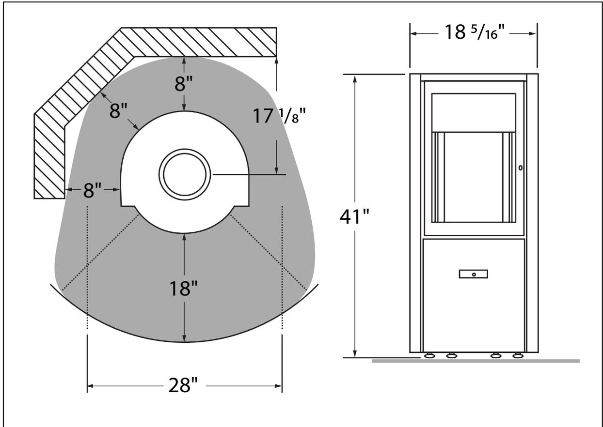
The clearances are indicated for all types of combustible materials (e.g.: wood, gypsum, etc.).
