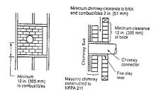
Minimum chimney clearance from masonry to sheet steet supports and combustibles 2 in, (\$1 mm)
