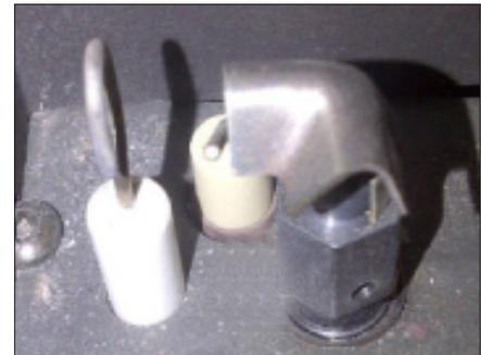
Figure 25: Correct Pilot Position
