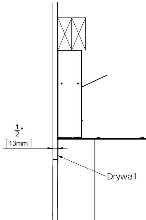
**Standard Thick Facing Install:** By adjusting the cabinet back, **non-combustible** material may be layered on top of the supplied Non-combustible board. Supplied board not needed for thick **non-combustible** finishes like rock.
