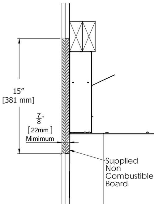
**Cool Surface System Extended Install:** By adjusting the cabinet back, **combustible** material may be layered on top of the supplied Non-combustible board. Supplied board is not needed for thicker **combustible** finishes.
