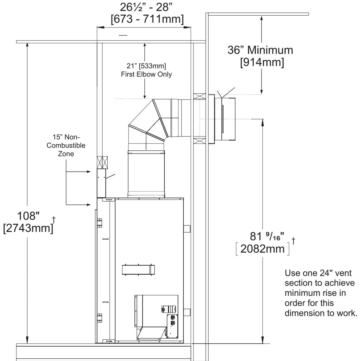
† Dependent of brand of 8x11 venting used. Additional 3" required if using Metal-Fab Sure Seal
