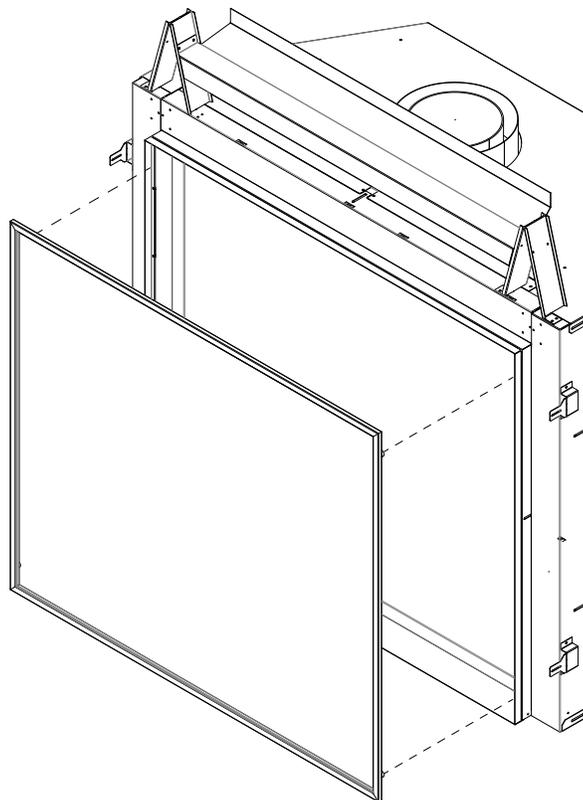
Figure 4: Safety Screen Removal
