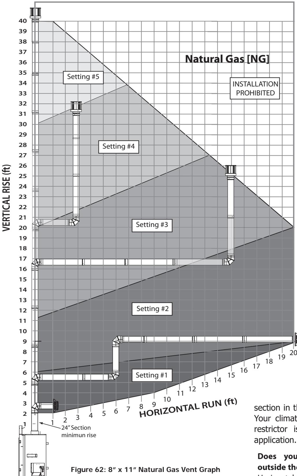
Figure 62: 8" x 11" Natural Gas Vent Graph
