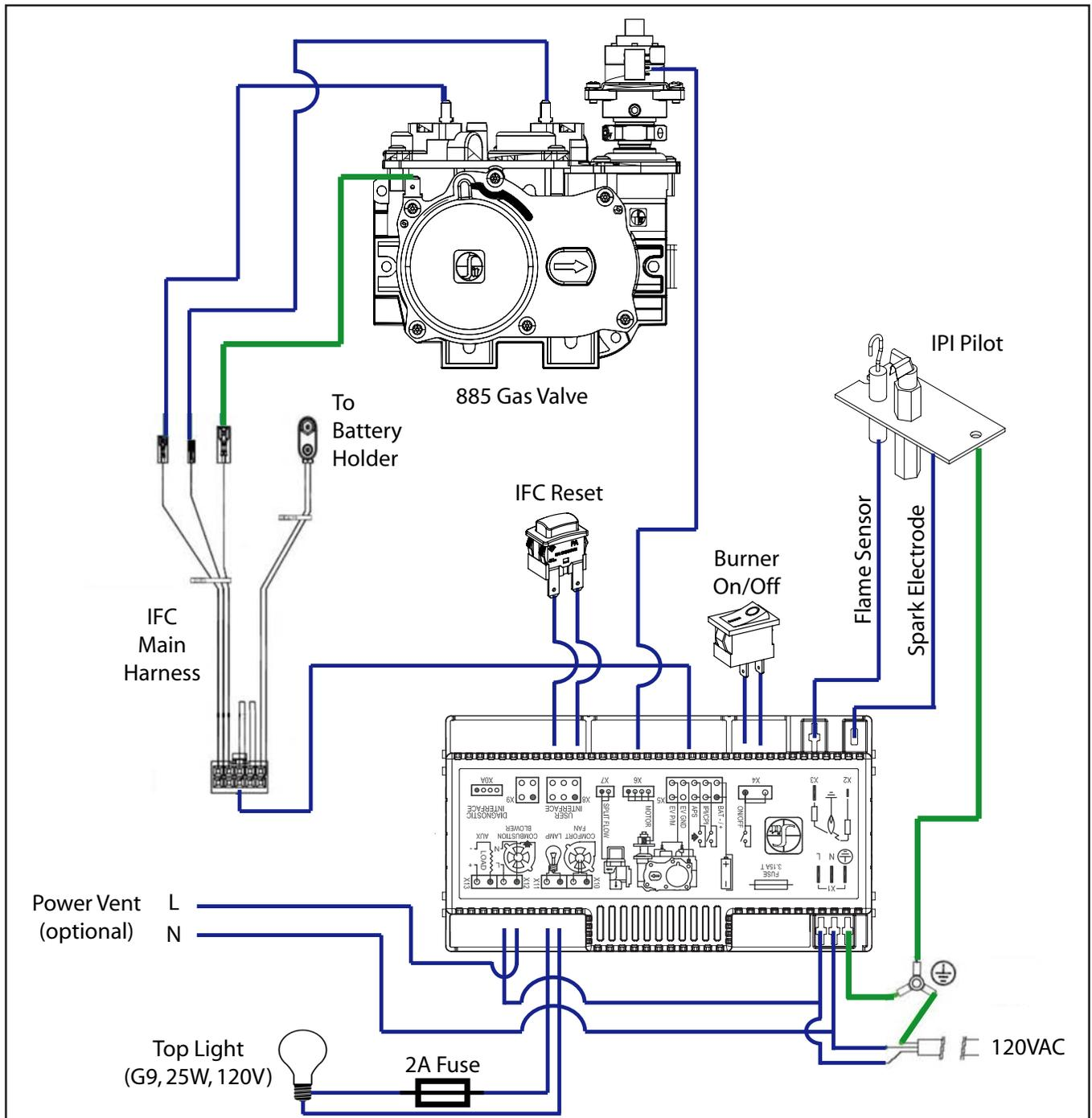
Figure 72: Wiring Diagram
