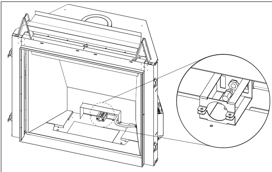
Figure 22: Orifice Location
