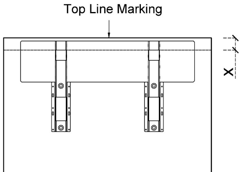
2. *Mount the Hanging Bracket:* Center the hanging bracket along the line marking made in Step 2. Using the information in the table below, mount the bracket to the wall using the four  $\frac{3}{8}$ "-diameter expansion bolts following the bolt manufacturer's requirements (bolts are not provided). Recommended bolt length is minimum 3" but may need to be longer depending on project design needs.
