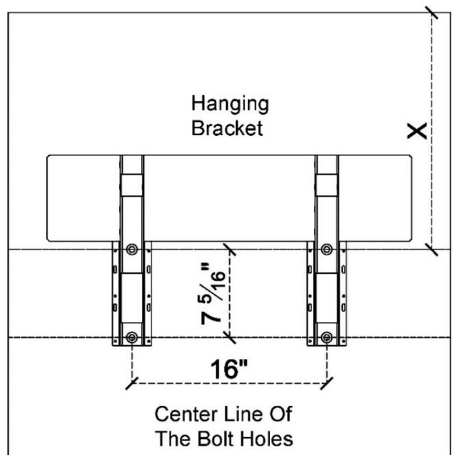
2. **Mount the Hanging Bracket:** Center the hanging bracket along the line marking you just made. Using the information in the table below, mount the bracket to the wall using the four  $\frac{3}{8}$ "-diameter lag bolts following the bolt manufacturer's requirements (bolts are not provided). Recommended bolt length is minimum 3" but may need to be longer depending on project design needs.
