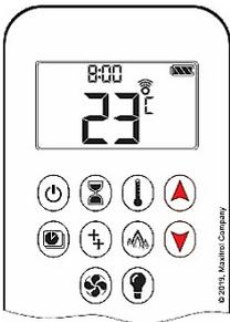
1. To increase flame height, press and hold the button to desired flame height.
