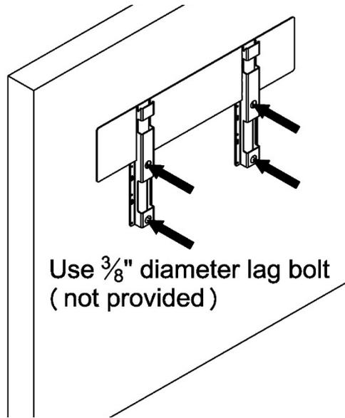
**NOTE:** To ensure the fireplace can be installed tightly to the wall, make sure the bolt doesn't stick out more than  $\frac{5}{8}$ " from the wall.
