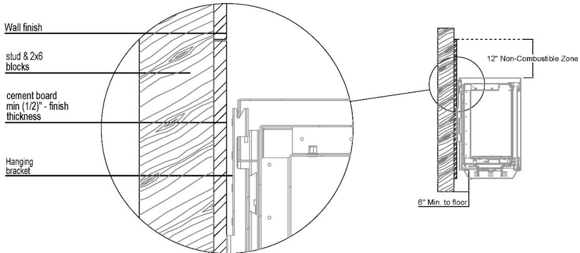
**! DIAGRAM NOTE:** The fireplace is shown in the diagram above as a reference point only. The fireplace will not be mounted to the wall until step 5.
