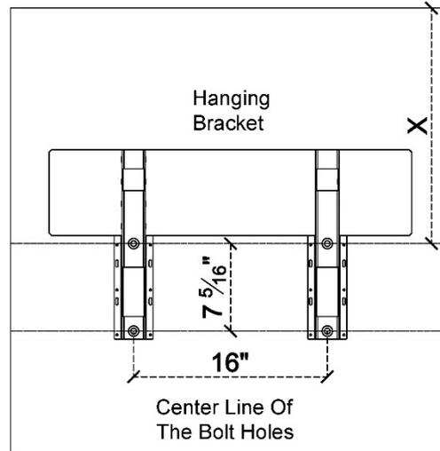
**! DIAGRAM NOTE:** The hanging bracket is shown in the diagram above as a reference point only. The fireplace will not be mounted to the wall until step 3.
