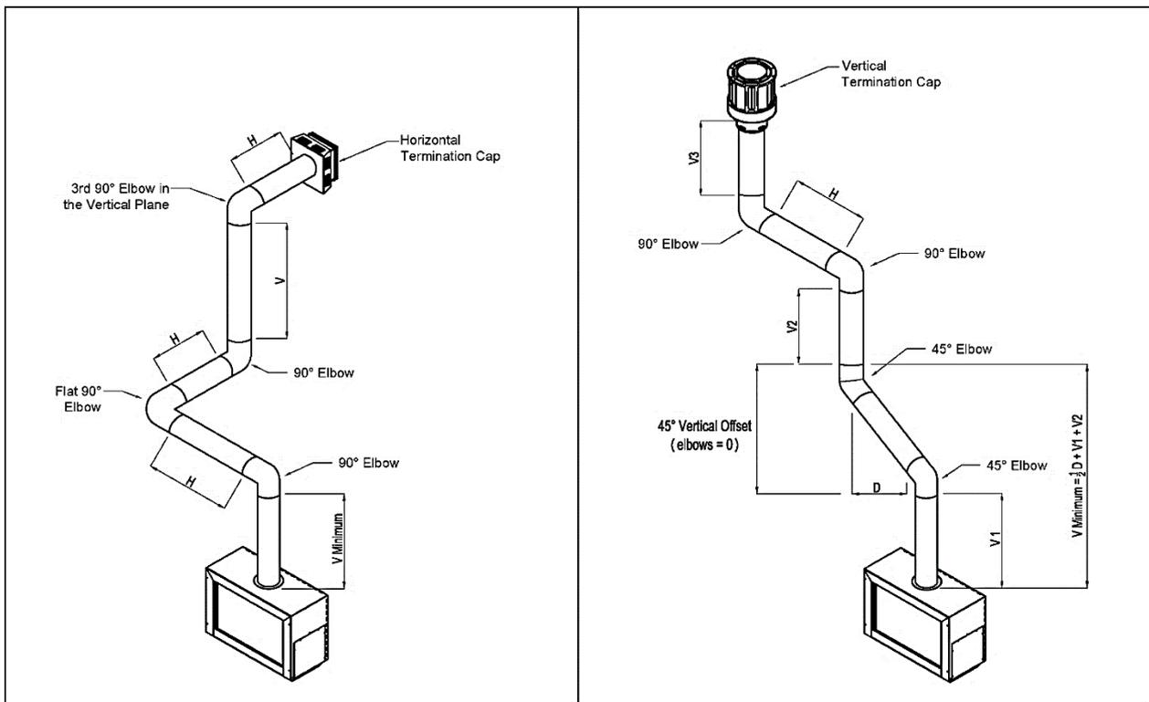
**! TERMINATION CAP NOTE:** Low Profile Termination Cap and Sconce Termination Cap can negatively impact flame appearance and are not recommended for use with the fireplace.
