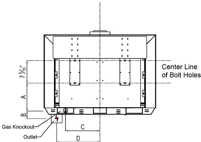
**A** = Distance from Center Line of Bracket Bolt Holes to the gas knockout.
