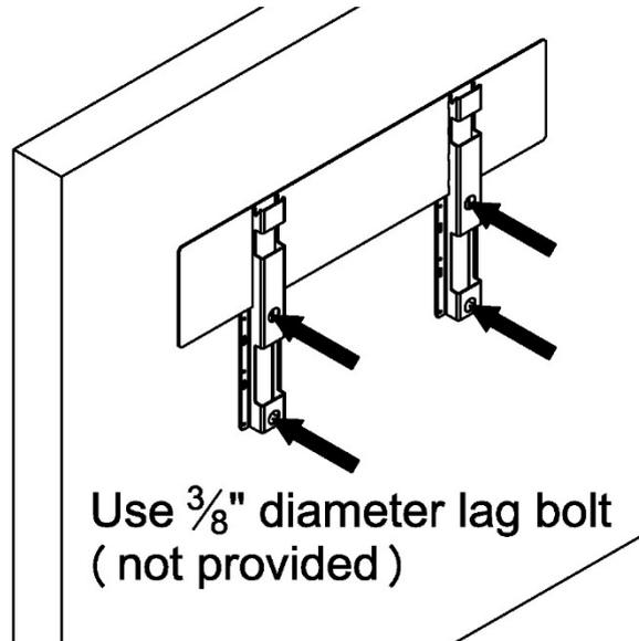
**NOTE:** To ensure the fireplace can be installed tightly to the wall, make sure the bolt doesn't stick out more than  $\frac{5}{8}$ " from the wall.
