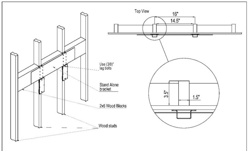
**! DIAGRAM NOTE:** The hanging bracket is shown in the diagram above as a reference point only. The hanging will not be mounted to the wall until step 3.
