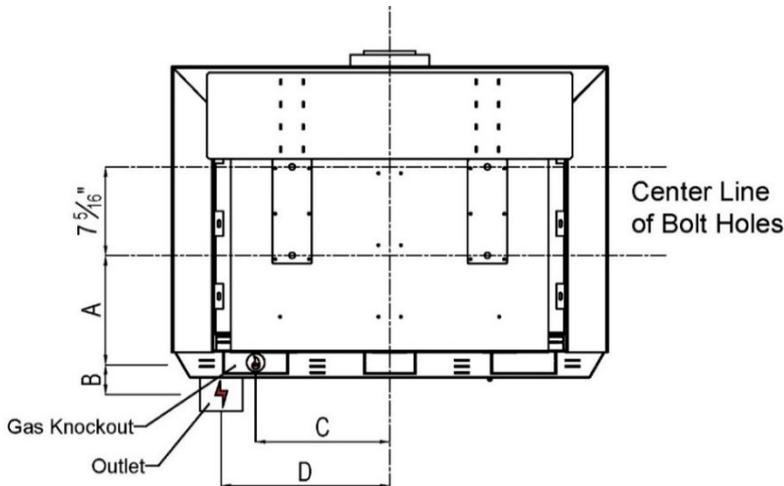
**A** = Distance from Center Line of Bracket Bolt Holes to the gas knockout.
