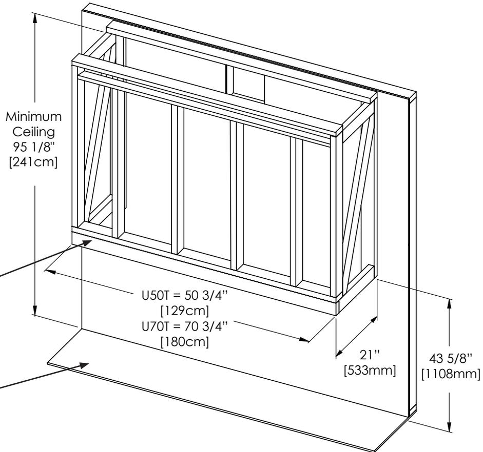
Maximum Front and Side Header depth = 1 1/2" (wood 2x4 on edge)
