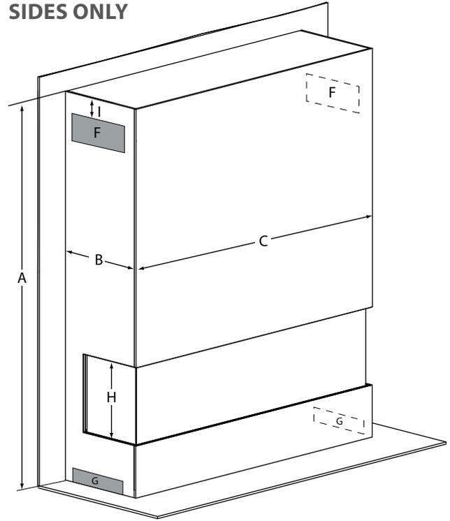
Heat release and intake on the sides of the chase only.
