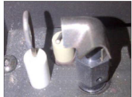
Figure 15: Correct Pilot Position
