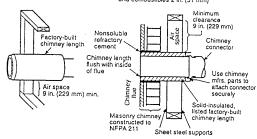
B Solid-insulated, listed factory-built chimney length of the same inside diameter as the chimney connector and having 1-in. or more of insulation with a minimum 9-in. air space between the outer wall of the chimney length and combustibles.
