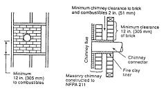
into combustible wall with a minimum of 12-in brick separation from clay liner to combustibles. The fireclay liner shall run from outer surface of brick wall to, but not beyond, the inner surface of chimney flue liner and shall be firmly cemented in place.
