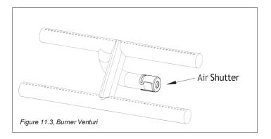
IMPORTANT: Slight adjustments to the venturi opening will create dramatic results. Adjust at slight increments until desired look is achieved. Always burn the fireplace for at least 15 minutes and allow the appliance ample time to cool before making any further adjustments.
