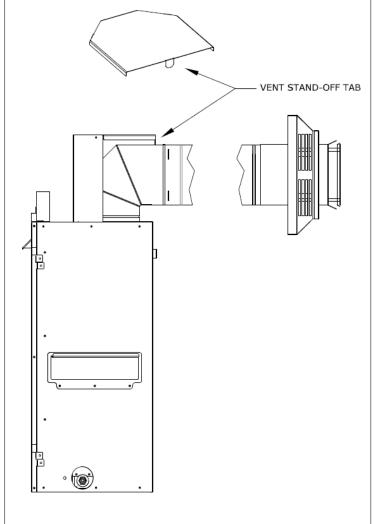
Figure 7.3, Installed Horizontal Heat Shield
