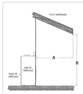
The overhang (A) must be a minimum of 1/2 or greater of the roofline elevation (B) above the base of the fireplace.
