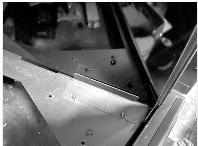
Figure 9.6, Black Glass Bottom Refractory Clip
