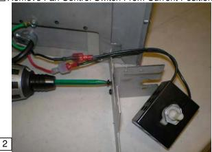
Attach Fan Control Switch Extension Bracket using [2] #6
