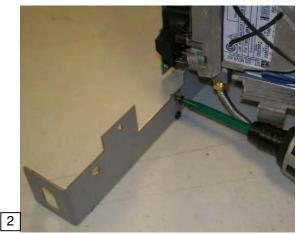
Attach On/ Off Switch Extension Bracket using [2] #6
