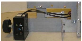
3 Mount Switch & route wiring as shown.
