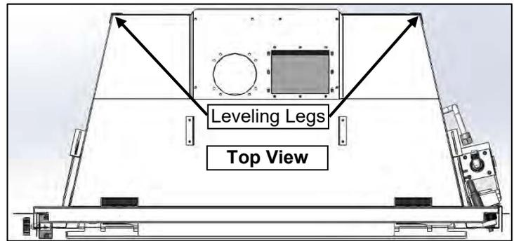
**IDV33 and IDV43:** There are two leveling legs at the front (for Flush Look installations) and two leveling plates at the back sides of the appliance. Remove screws and set to proper height. Replace screws.
