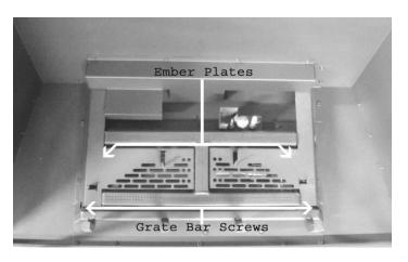
Remove the ember plates and the grate bar by removing the 2 left and right screws on the grate bar. Reinstall screws after removing parts.
