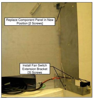
3. Install Component Panel and Fan Switch Extension in new position.
