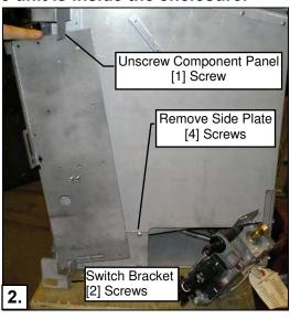
Remove Component Panel, Switch Bracket, and Side Plate.
