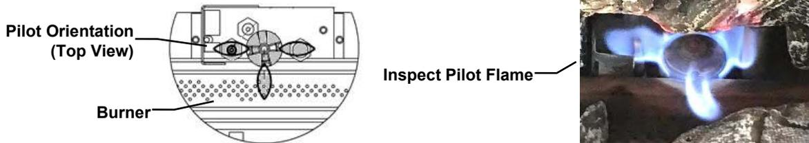
4. Inspect and ensure the lighting of the main burner occurs within 4 seconds of the main gas valve opening. Visual inspection should match that outlined in the appliance instruction manual (refer to **Monthly Flame Inspection**). Inspect primary air openings for blockage.
