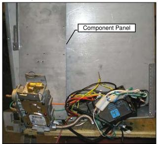
Remove All Components from Component Panel.
