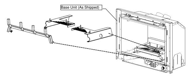
Preparation: Remove Grate Bar and replace screws. Remove Ember Plates. Do not remove existing Pilot Shield.
