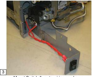
Mount Switch & route wiring as shown.
