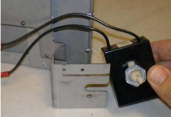
**1** Remove Fan Control Switch From Current Position.
