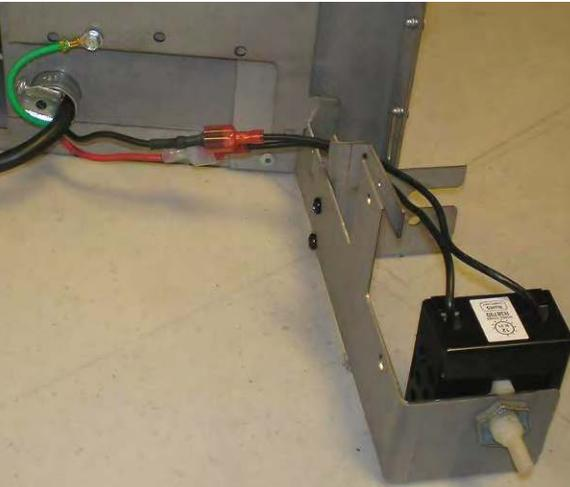
**3** Mount Switch & route wiring as shown.
