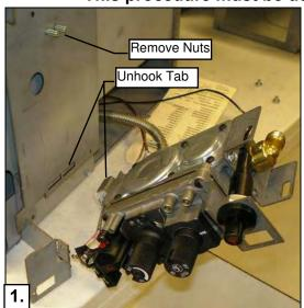
Remove [2] 3/8" nuts holding valve onto Component Panel. Unhook valve from Component Panel.
