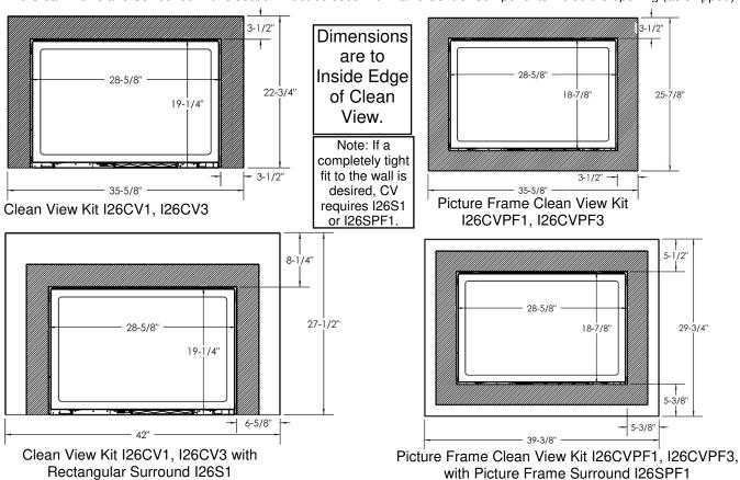
\*The Clean Views in this section can be used with Valve Control Components inside or outside the opening, HOWEVER-if controls are outside, these Clean Views MUST be used to cover valve controls.
