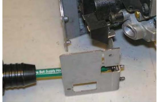
**1** Remove On/Off Switch and original mount bracket.
