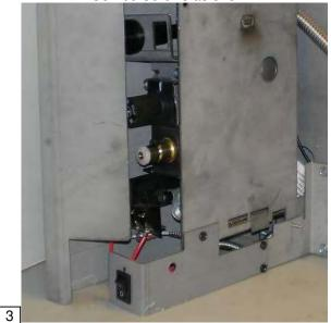
Mount Switch & route wiring as shown.
