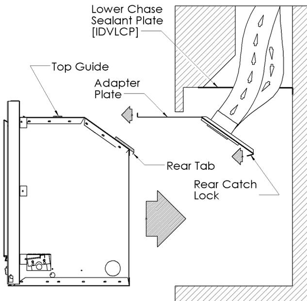
Fig. 2 - Base unit chimney venting install.
