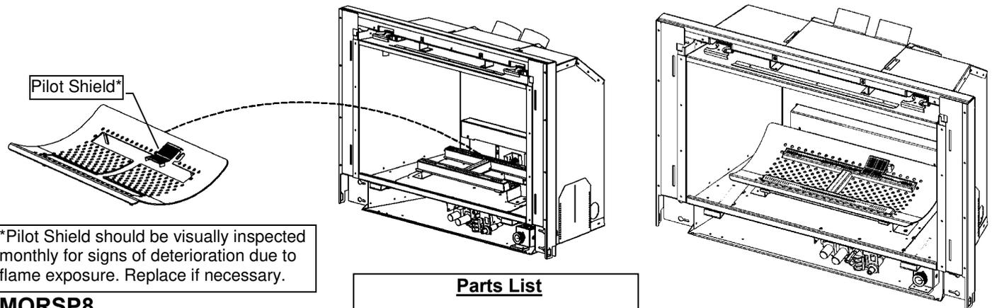
\*Pilot Shield should be visually inspected monthly for signs of deterioration due to flame exposure. Replace if necessary.
