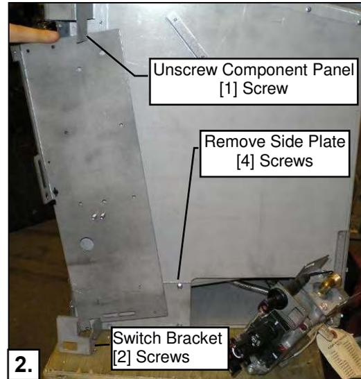
**2.** Remove Component Panel, Switch Bracket, and Side Plate.
