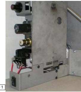
Remove On/Off Switch and original mount bracket.
