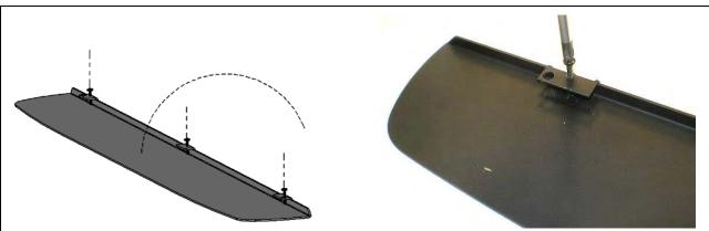
Place I33CS upside down on a protected surface. Loosen screws.
