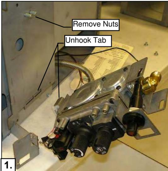
**1.** Remove [2] 3/8" nuts holding valve onto Component Panel. Unhook valve from Component Panel.
