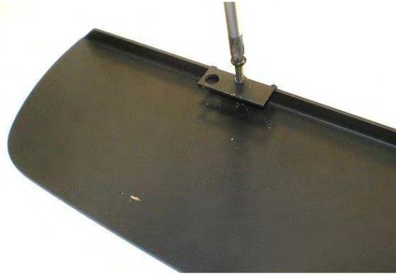
Place I33CS upside down on a protected surface. Loosen screws.
