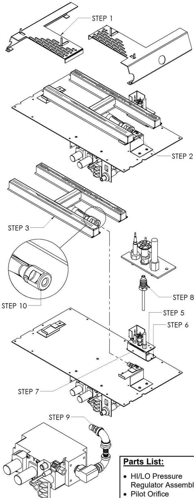
1. Remove the 2 ember plates from the burner. This step may not be required, depending on the type of burner assembly.
