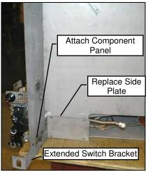
Replace Side Plate. Attach Component Panel and Extended Switch Bracket.
