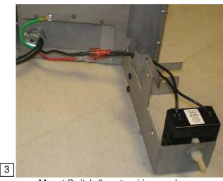
Mount Switch & route wiring as shown.
