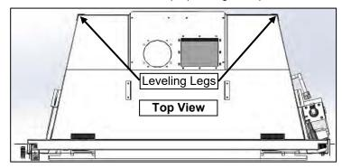
**IDV33 and IDV43:** There are two leveling legs at the front (for Flush Look installations) and two leveling plates at the back sides of the appliance. Remove screws and set to proper height. Replace screws.
