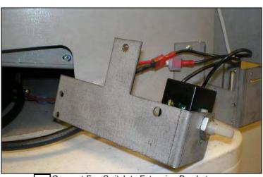
2 Connect Fan Switch to Extension Bracket.
