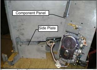
Remove Side Plate and knockout if present (see millivolt section). Place Component Panel on other side of valve.
