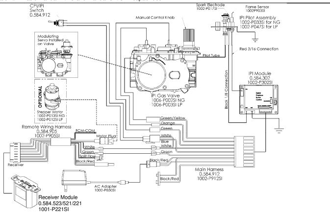
Configuration #2: Remote ON/OFF and manual HI/LO capabilities. OPTIONAL: For units with remote HI/LO capabilities, a modulating servo is required to be installed on the valve. The connectors to this servo must be connected to the Remote Harness as shown in the figure above.
