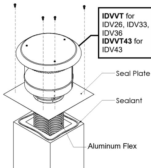
**Installation of Vertical Termination**
