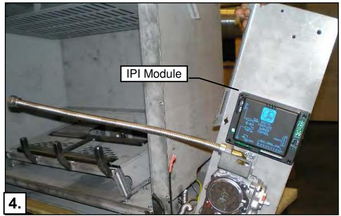
4. **Optional-** Connect flex (Not included. Order PN# **FP15GC**) to inlet side of valve. This can then be connected to the gas supply and routed through the channel inside the fireplace. (see millivolt section).
