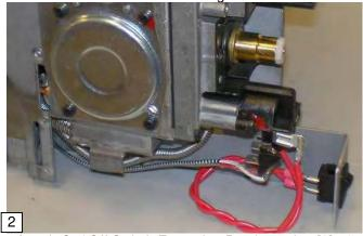
Attach On/ Off Switch Extension Bracket using [2] #6
