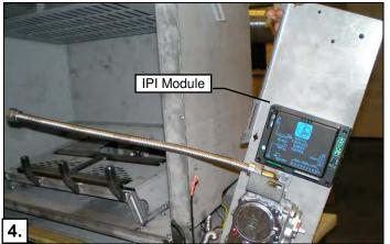
**Optional-** Connect flex (Not included. Order PN# **FP15GC**) to inlet side of valve. This can then be connected to the gas supply and routed through the channel inside the fireplace. (see millivolt section).
