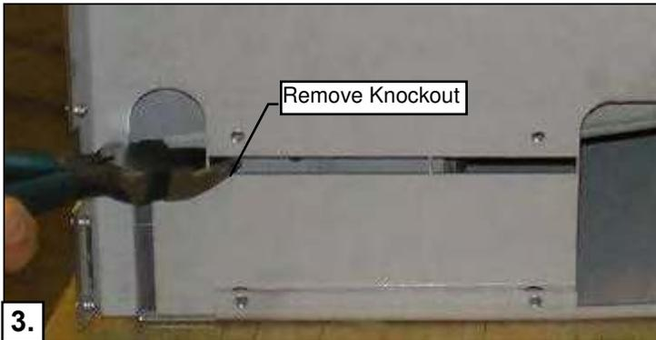
**3.** Remove knockout with side cutters, if present. Discard knockout.
