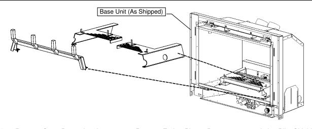
**Preparation**: Remove Grate Bar and replace screws. Remove Ember Plates. Do not remove existing Pilot Shield. **Installation**: Install RSP10 by placing over burner. Use existing screws at front of firebox bottom to attach Glass Retainer.
