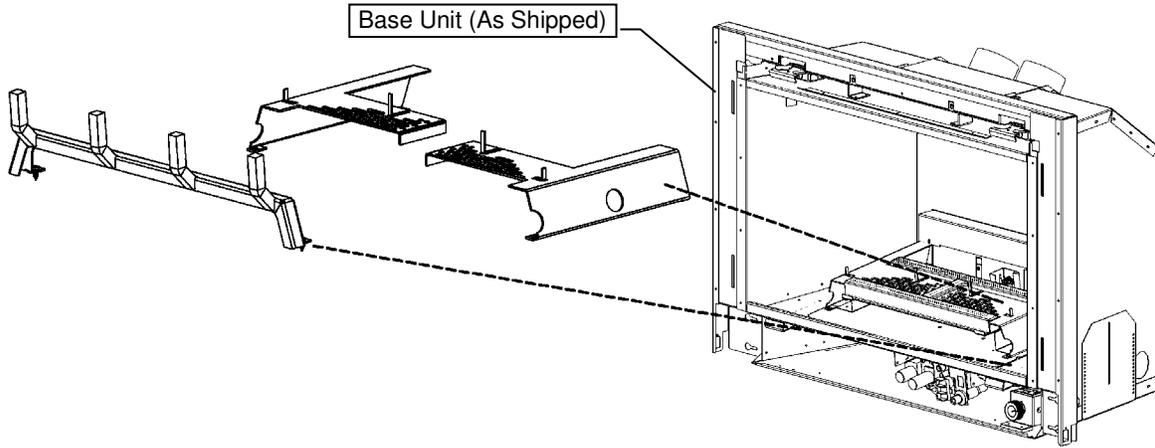
**Preparation:** Remove Grate Bar and replace screws. Remove Ember Plates. Do not remove existing Pilot Shield.
