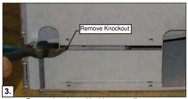
Remove knockout with side cutters, if present. Discard knockout.
