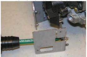
1 Remove On/Off Switch and original mount bracket.
