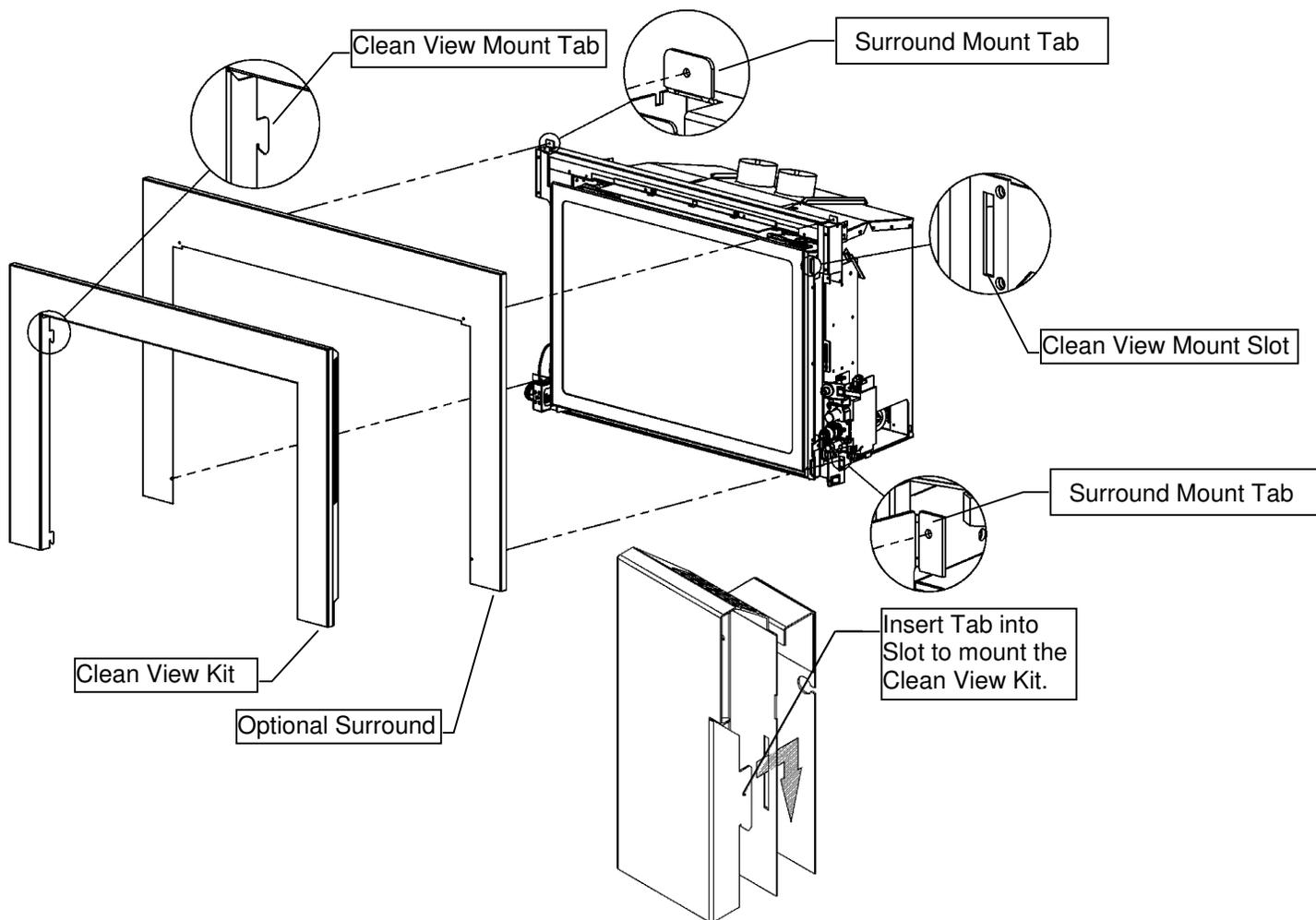
**NOTE: The Clean View Surround needs to be removed in order to access the Glass Door, access the valve, and service the unit.**
