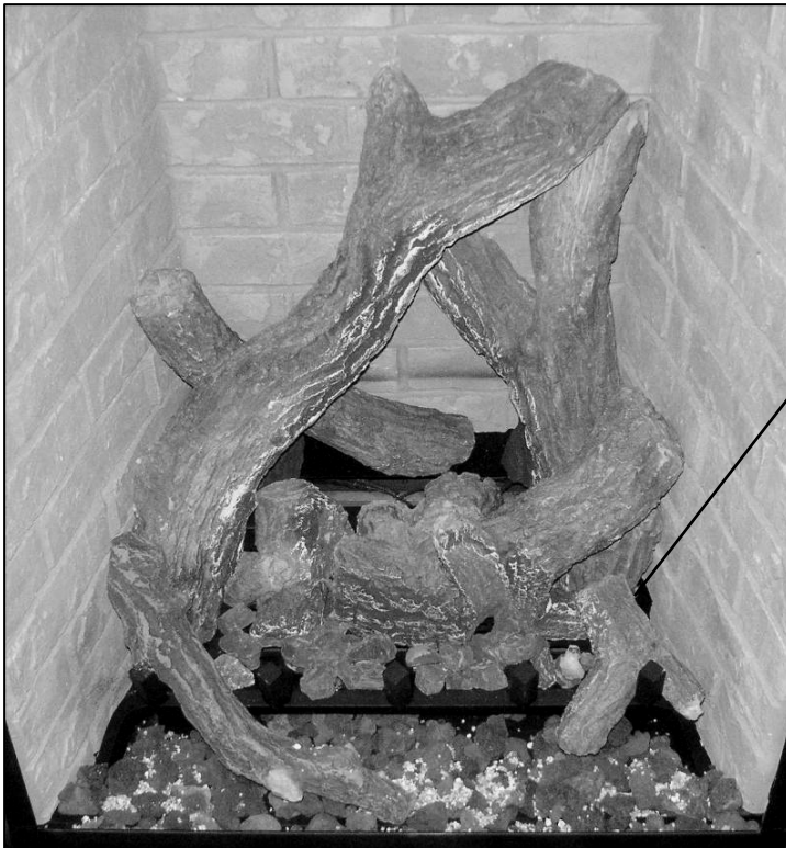
Step 6: Add lava rock to the bottom of the burner pan. Add glowing embers to the top of the ember plates and front burner tube. And sprinkle vermiculite over the lava rock. Do not place any media within Pilot Shield Area (see above).
