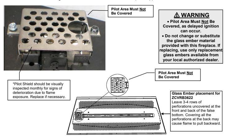
NOTE: Glass Media must be evenly spread over the Burner and False Bottom as described on last page before Rock / Stones / and Log Accessories are placed.
