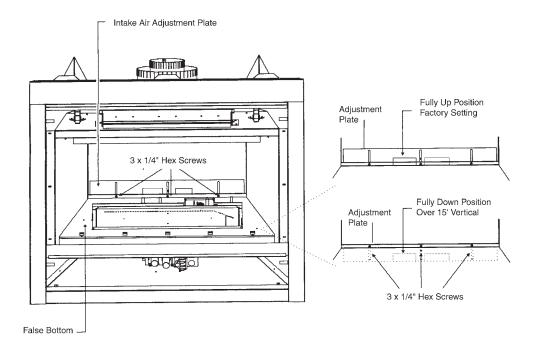
NOTE: Unit comes preset for short horizontal or vertical venting under a 15 feet run.
