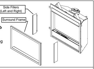
1. With Glass Door removed, hook Surround over Lower Ledge of fireplace and slide Side Fillers into place.
