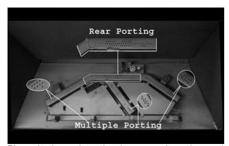
Place glowing rock wool on burner as shown in step 1 being sure to leave the multiple porting areas open. For Lp only, the multiple porting areas can be completely covered. Do not cover the Rear Porting areas with rock wool.
