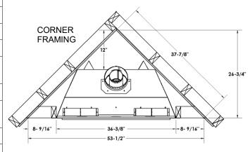
Framing for Horizontal Vent Termination (See Installation of Side Wall Venting Section)
