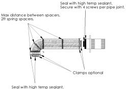
Seal with high temp sealant. Secure with 4 screws per pipe joint.
