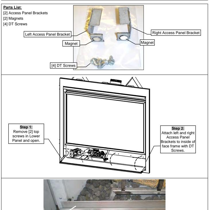
Step 2 (illustrated): Install screws in top corners. Attach left and right Access Panel Brackets to inside of face frame with DT Screws. Lower Face Panel will now be openable.
