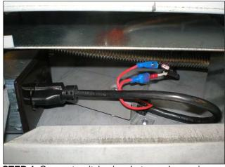
**STEP 4**: Connect switch wires between lamp wire and transformer (see schematic). Connect remaining lamp wire to transformer. Transformer can then be plugged in and the housing fastened to the bottom of the fireplace.
