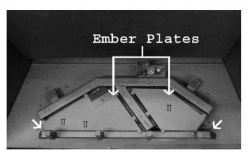
Step 1: Remove the grate bar by removing the 2 Screws located on the left and right side of the grate bar as illustrated. Remove the 2 ember plates once the grate bar is removed. The 2 screws removed must be re-installed once the grate bar is removed.
