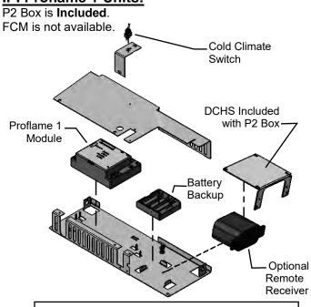
NOTE: BATTERY BACKUP PACK IS NOT REQUIRED IF REMOTE RECEIVER IS USED
