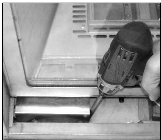
Power Vent Control Module Mounted inside fireplace.
