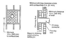
Minimum chimney clearance from masonry to sheet steel supports and combustibles 2 in, (\$1 mm)
