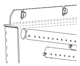
Align and insert the notch into the hole on the other side
