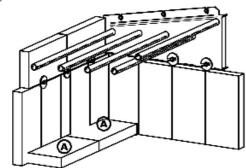
6) After, insert 4 bricks «A» in front of the 2 bricks previously installed.
