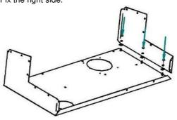
4) Attach the front part (with the door) to the two sides and the back. Keep the horizontal holes for the chrome decoration.
