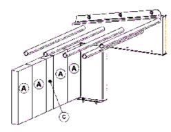
2) Set the 3 big screws in the holes for this purpose. Do not tighten up these screws too much, so that washers will be easily installed.
