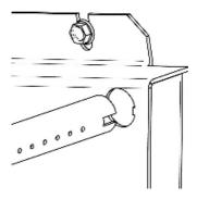
3) Push completely the notched end and insert the cotter pin into the last hole on the other side.
