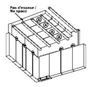
3) Put the rockwool over the bricks and verify from the holes on the collar of the chimney to make sure the smoke exit is not obstructed.
