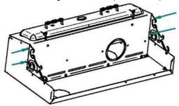
Fix the top with the back and the front. Do not fix the chrome head now.
