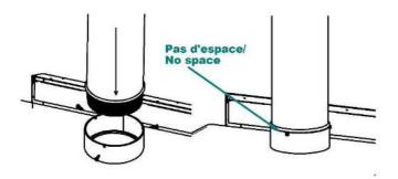
WARNING: It is mandatory to attach the pipe to the stove collar and also at each joint with at least of 3 screws.
