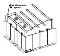
Place 4 bricks « A » over the two front pipes. It must be placed as shown in the picture below. Be sure to leave no space in between the bricks previously placed.
