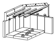
7) Insert 1 brick «A» on the right of the ash dump plug. 8) Insert 1 brick «B» on the left of the ash dump plug.
