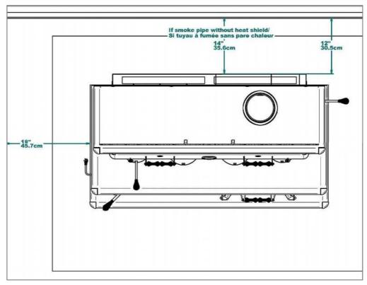
For a 45° corner installation, or other corner installation, the minimum clearance between the cook stove and combustible material must be 18 inches.
