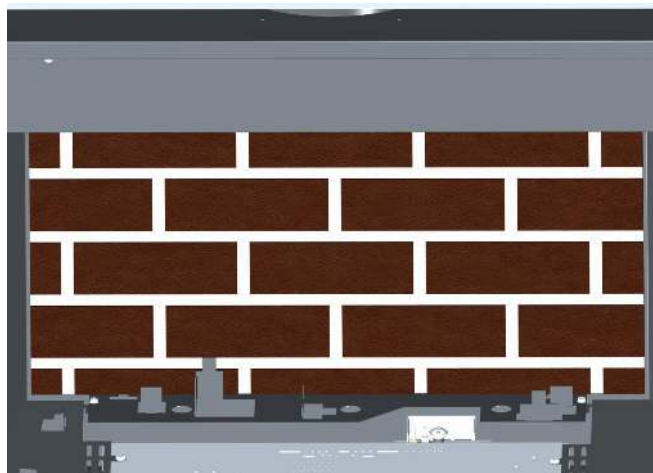
Figure 39A - Install Rear Fiber Panel
