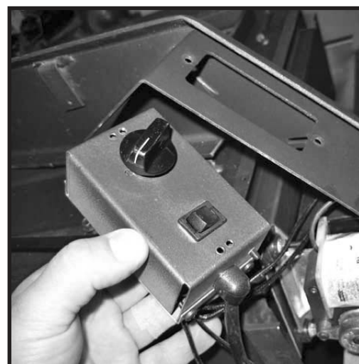
Figure 17: Removing speed control assembly.
