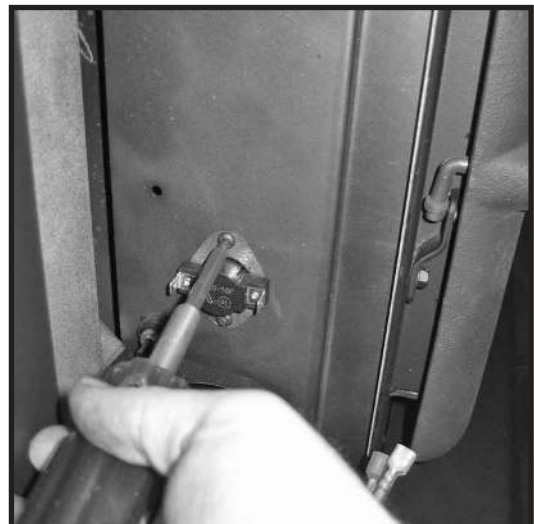
Figure 23: Relocating thermal switch to left side.
