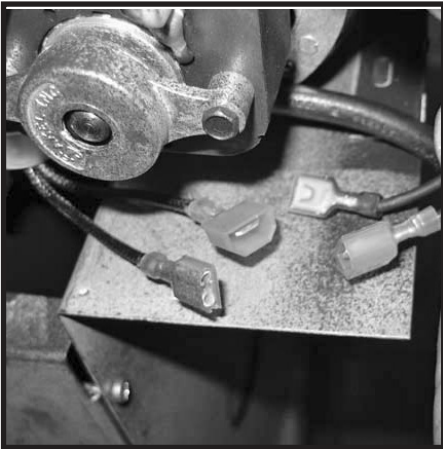
Figure 15: Disconnecting fan wires.
