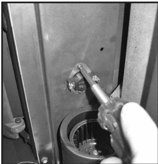
Figure 22: Removing thermal switch.
