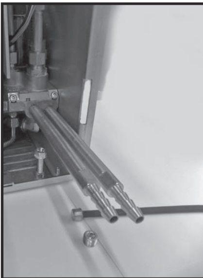
Figure 41: Gas valve location.
