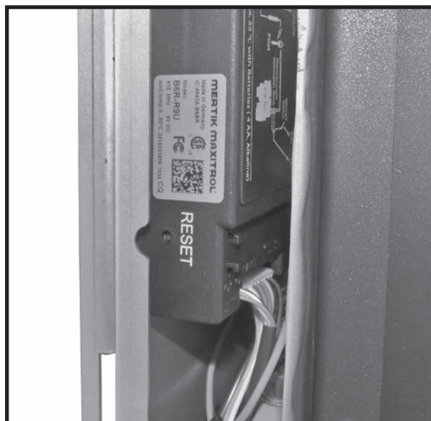
Figure 98: Maxitrol reset button location.
