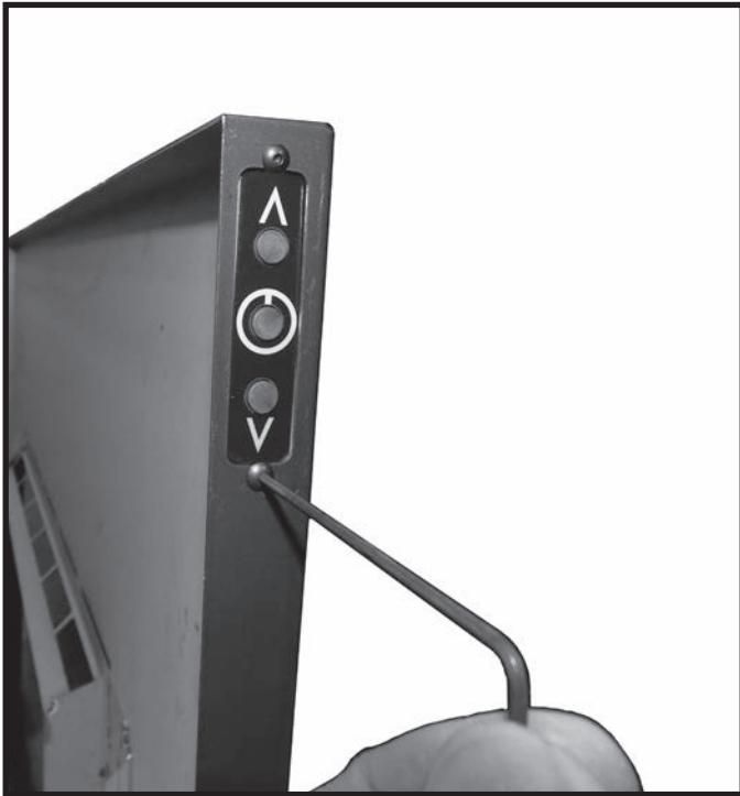
Figure 91: Attaching switch to backing plate.
