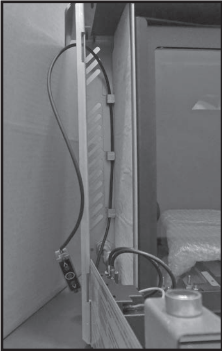
Figure 88: Pre-installed ON OFF switch assembly.
