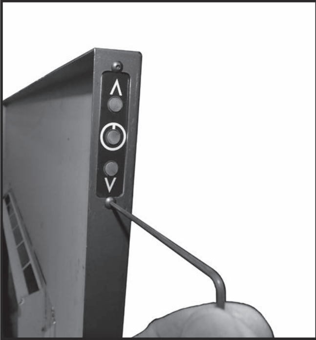
Figure 108: Attaching switch to backing plate.
