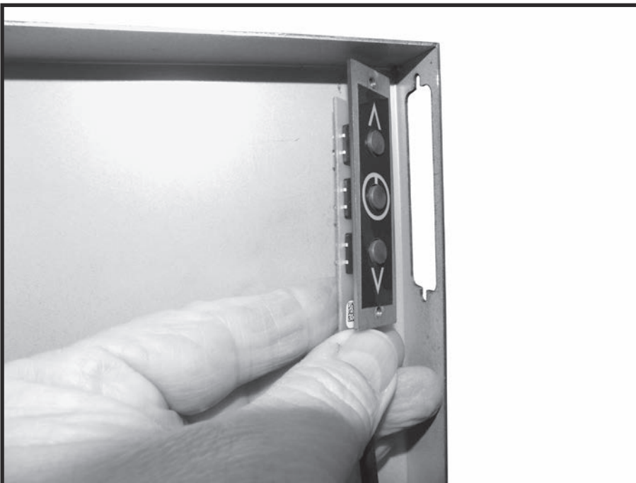
Figure 107: Positioning the switch behind the backing plate opening slot.
