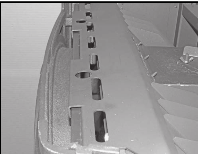
Figure 61: Screen holder in correct position.
