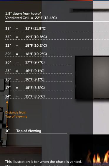
This can be done by either installing a grill on the front or sides of chase (for a chase that bumps out into a room) or be open at the top of the chase. (See installation manual for further information).
