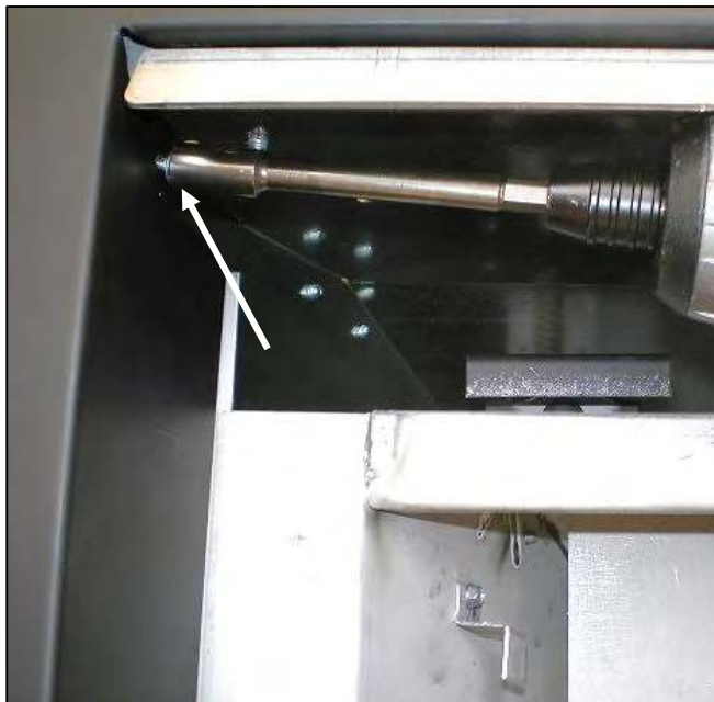
Step 3 (illustrated): Install screws in top corners.
