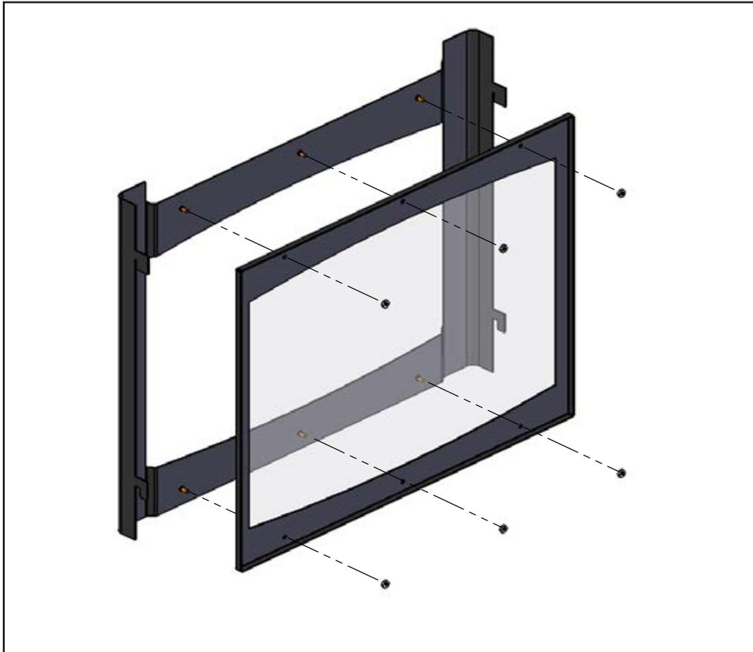
**Figure 71: Safety Screen Removal**
