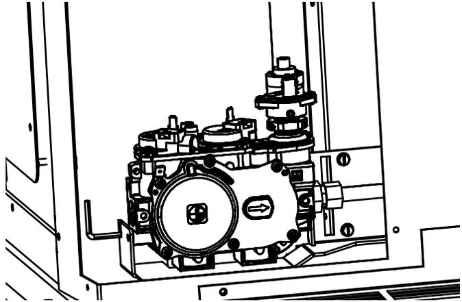
Figure 3: Gas Valve In Place on Unit.
