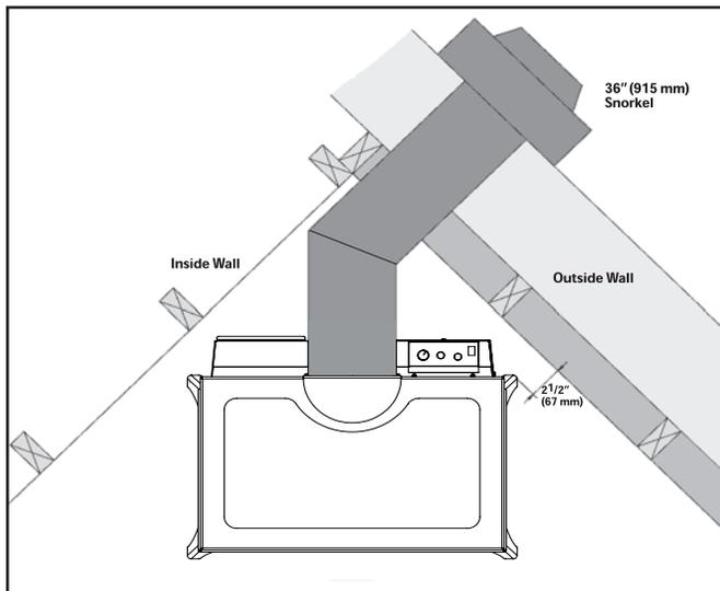
Figure 41: Corner installation rear vented with snorkel.
