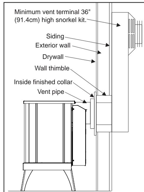
**Figure 46: Installation for Rear Vented; 30,000 Btu/hr.**
