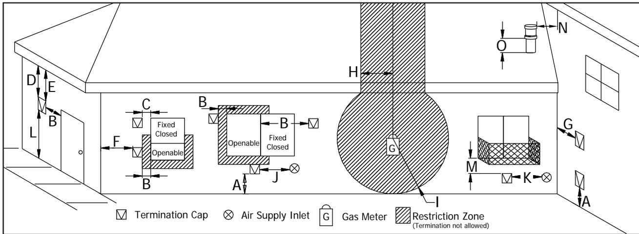
Figure 26. Vent Termination Restrictions, refer to Table 3.
