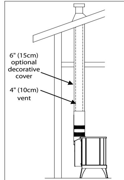
Figure 52: Unit top venting styles.
