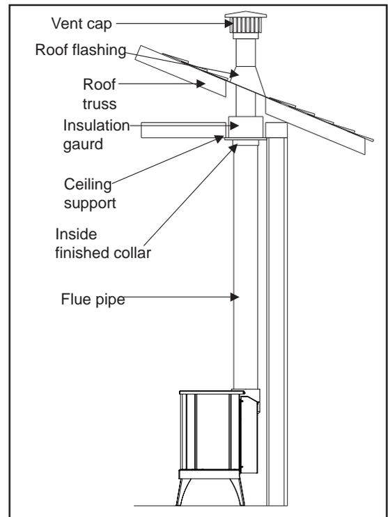
**Figure 48: Installation for Top Vented; Vertical Termination.**
