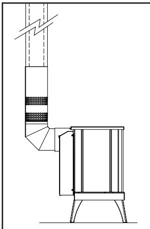
Figure 53: Unit rear venting style.
