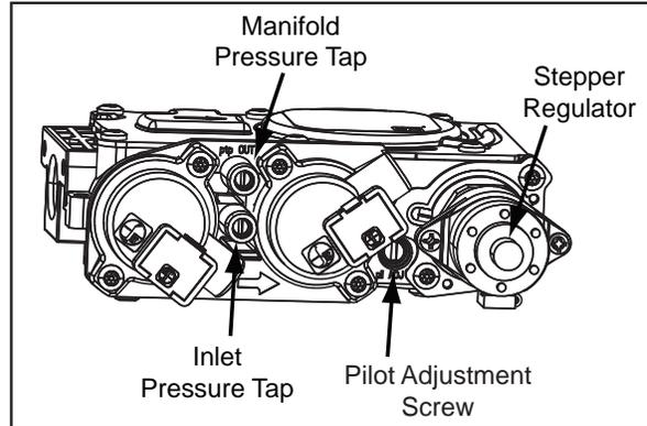
**Figure 56: Fully Labeled Gas Valve.**
