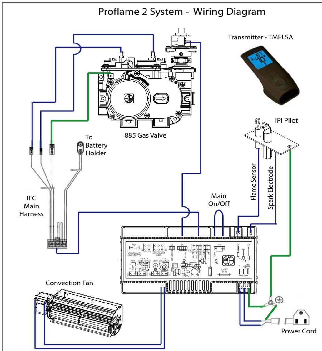
Figure 57: Wiring Diagram
