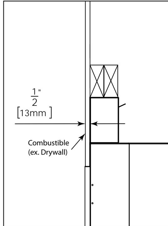
**Standard Extended Install:** Using the supplied long finishing edge, **non-combustible** material may be layered on top of the supplied Non-combustible board. Supplied board not needed for thick **non-combustible** finishes like rock.
