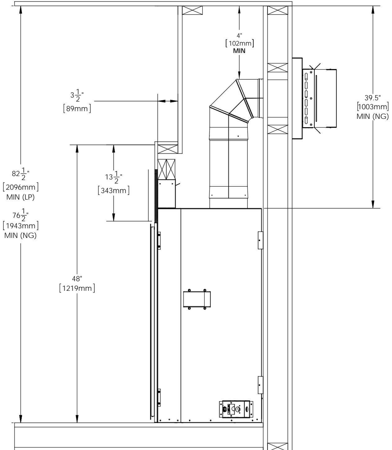
Figure 45: Recess Installation
