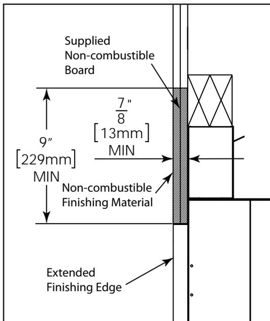
**Cool Surface System Extended Install:** Using the supplied long finishing edge, **combustible** material may be layered on top of the supplied Non-combustible board. Supplied board is not needed for thicker **combustible** finishes.
