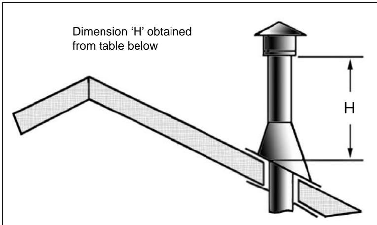
**Figure 63: Height of Vertical Termination; Reference Table 8**
