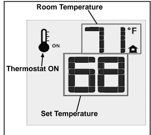
Figure 8: Thermostat Function
