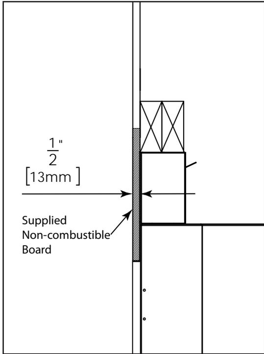
**Cool Surface System (CSS) Install:** Image shows the short finishing edge, **combustible** can be brought right down to the finishing edge.
