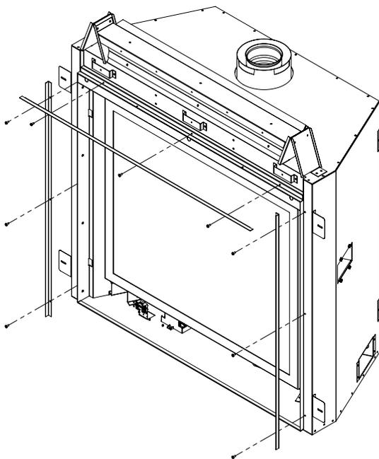
Figure 30: Outer finishing edge removal / replacement
