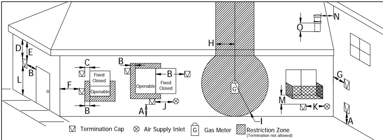
Figure 55: Vent Termination Restrictions, refer to Table 4
