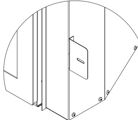
Figure 27: Nailing Flange Assembled
