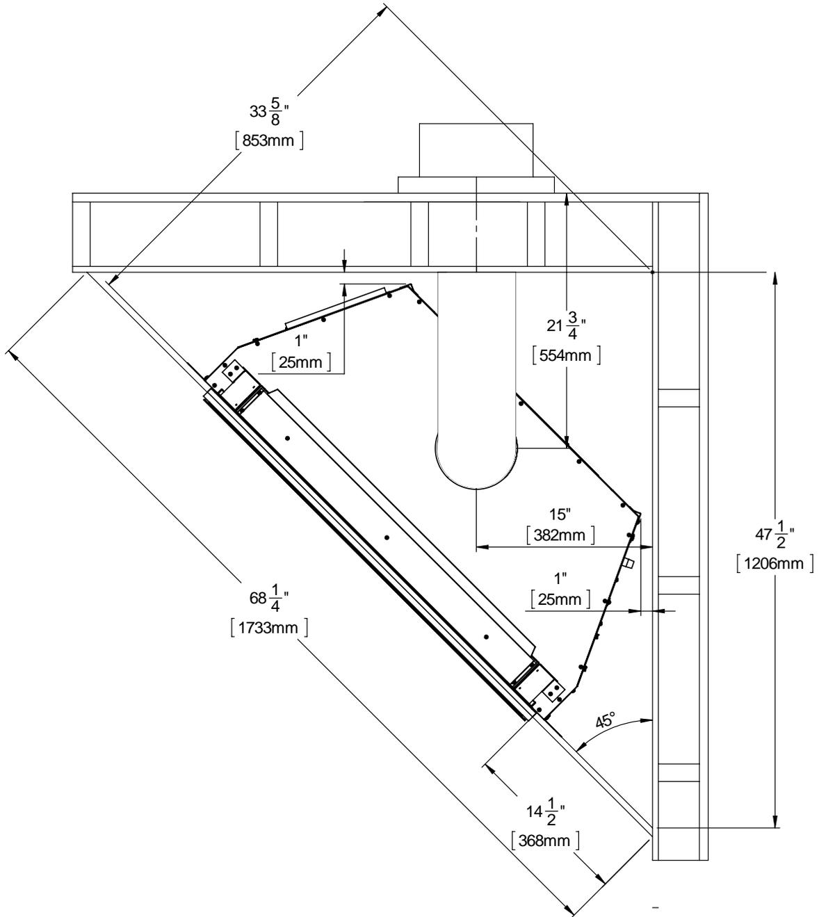
Figure 46: Corner Installation
