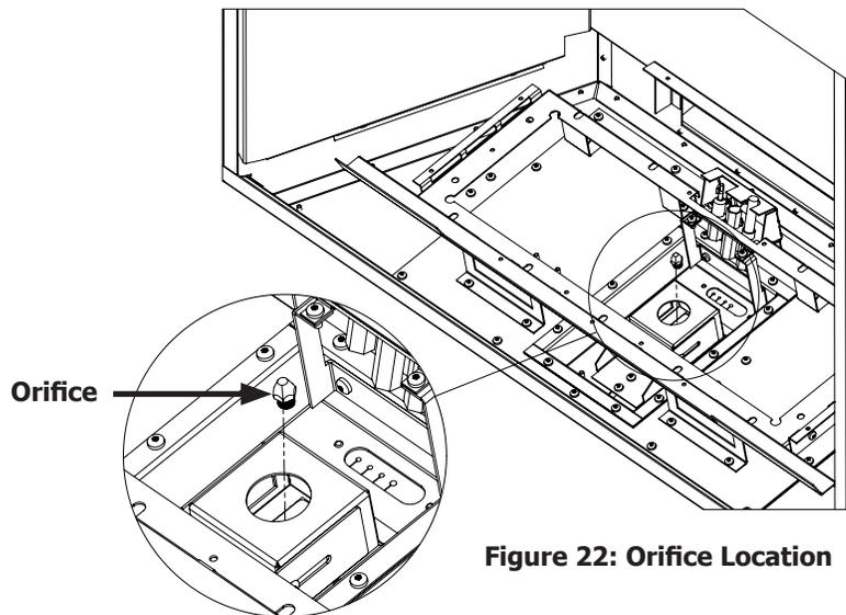
Figure 22: Orifice Location
