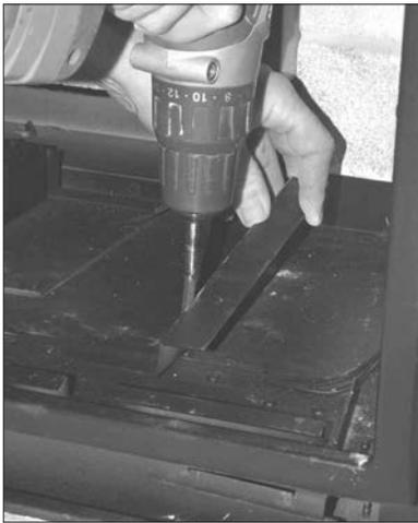
**Figure 56: Removing the Right Burner Support.**
